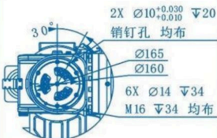
末端法兰安装尺寸 End flange mounting size
